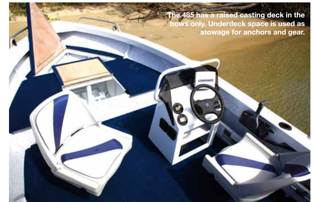
The Sea Jay 485 Haven has higher sides than most of its genre and the inherent toughness of “plate” aluminium construction.
