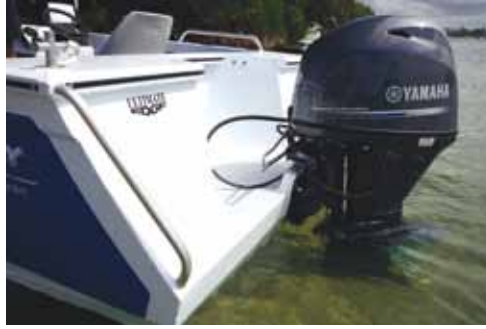
Transom offers the safety of a full height aft bulkhead.
